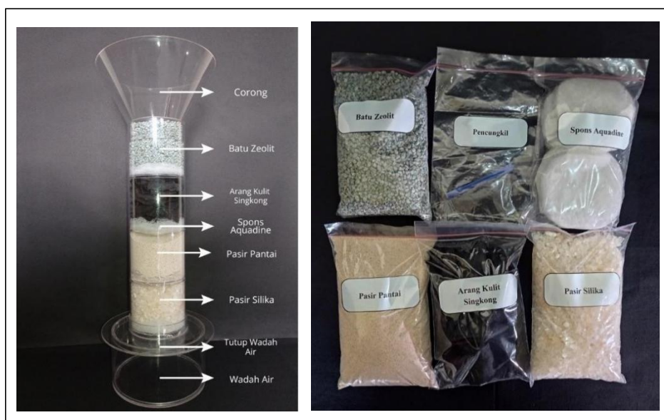
Figure 2. Realization of the STEM KIT Water Filter Design (Left: Water Filter; Right: Water Filter Media)
